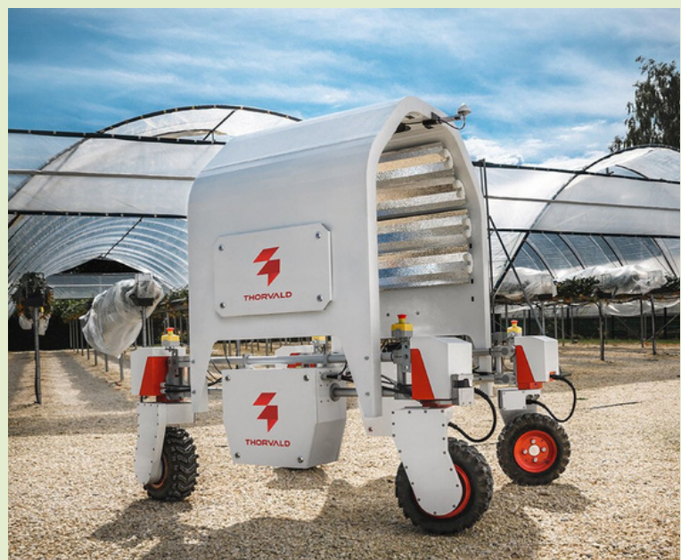
Autonomous crop protection – the Thorvald-Saga Robotics UV application machine
