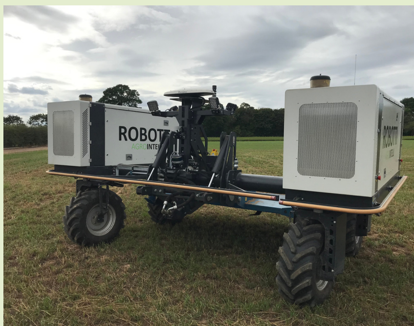
Agointelli Robotti autonomous platform which can be linked to various pieces of cultivation equipment
