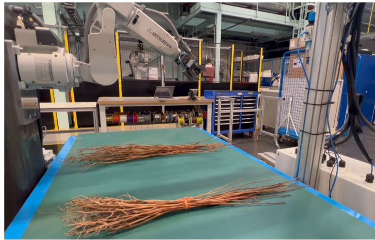
Singulation of plants by the robot arm
