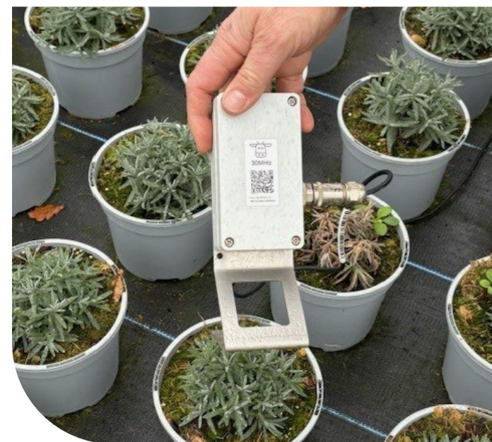
Example 1. The probe used to understand water levels, humidity conductivity and temperature to ensure optimum growing conditions.
