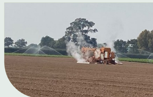
Example 3, GPS guided fully autonomous steaming machine that kills pathogens in soil at 85 degrees Celsius.
