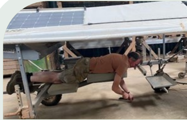
Example 1, Solar powered weeding machine allowing the picker to lie down and avoid bending.
